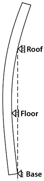
Prestress-induced camber (exaggerated) with an intermediate floor connection and a parapet.
